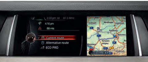
BMW's iDrive 4.2 Navigation system guides you to your destination, which is displayed on a high-resolution 10.2-inch screen. The 200 GB hard-drive-based system features include 3-D daytime and nighttime maps, zoom and satellite images, travel planner, and a split-screen view. It also offers Voice command for convenient, hands-free operation, and 20 GB of storage for your favorite media files. Advanced Real Time Traffic Information (ARTTI) displays and describes current local traffic information on your Control Display. In case of delays greater than five minutes, it suggests alternate routes.
