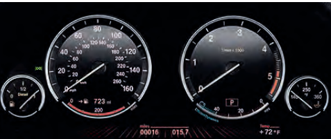
Black Panel Display shows a matte black surface when the ignition is off, with only the chrome rings of the circular instruments visible in 3-D. Switched on, the graphics display lights up, showing the trip computer and Check Control information; below the four analog dials is a high-res, wide-format Info Display that shows Navigation instructions, music tracks, etc. When ECO PRO mode is active, ECO PRO tips use graphics to encourage a more efficient driving style.
