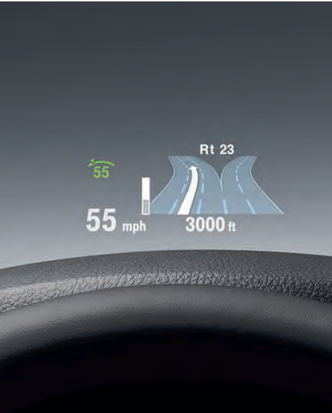
Head-up Display projects important travel information, such as current speed and Check Control data, on the windshield directly in your line of vision in full color. Also displayed are directional arrows from the Navigation system, Speed Limit Info, and other driving warnings, as well as radio stations, music and phone lists.
