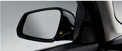
Lane Departure Warning , 2 one of the features of Active Driving Assistant, senses when your vehicle is crossing over roadway lane markings or is changing lanes without signaling, and warns you by sending a mild vibration through the steering wheel. The system can be turned on and off via a button near the steering wheel.
