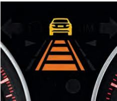
Active Cruise Control with Stop & Go 2 lets you preset desired speed and following distance. When it recognizes slower vehicles ahead, it reduces your speed to maintain the preset distance, and can even bring you to a complete stop if traffic calls for it. Active Cruise Control also includes the Active Driving Assistant features.
