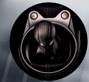
**A world's first.** Included on the Sport models, SynchroRev Match® technology – the first in any production car – monitors the 6-speed manual's clutch pedal, shift lever, and vehicle speed. As you shift to a lower gear, the system will “blip” the throttle to the ideal engine rpm for a supremely smooth downshift as you let out the clutch. The system also works when upshifting to give you a smooth flow of power when accelerating.
