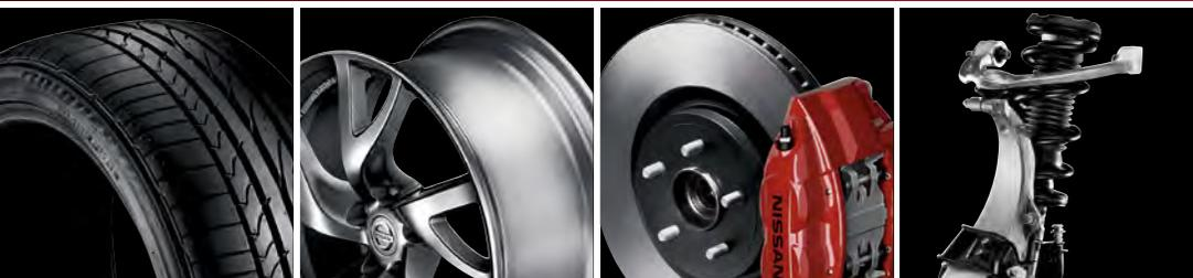
**Lightweight suspension components.** The lighter a suspension's components, the more quickly it can react to the driver and bumps in the road. Use of strong yet lightweight aluminum makes the Z<sup>®</sup> suspension extremely responsive. Its double-wishbone front and 4-link rear design helps to keep the tires vertical to the ground, maximizing their contact patches. Dual flow pass shocks enhance control. And super-light forged 19" alloy wheels are available for even quicker response.
